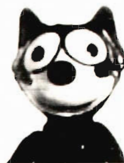
Improved definition is obvious to anyone in this all-electronic 120-line image of Felix—transmitted in the early days of NBC television.
